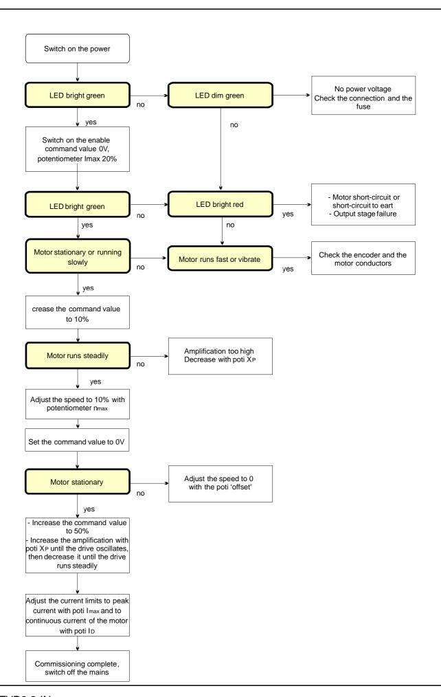
Functional diagram bl/ec motor amplifier
